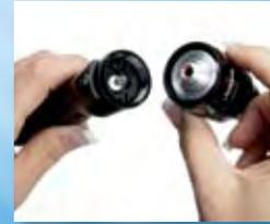
When the bulb is cool pull it out of its socket.
