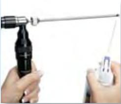
If the mirror is still soiled, lightly dampen a cotton swab with Hawkeye lens cleaner, isopropyl alcohol or acetone. Hawkeye lens cleaner works well on fingerprints and dust...use acetone on oil or grease. Gently clean the mirror with the fewest strokes necessary, taking special care not to drag debris across the mirror surface. Lightly wipe with a dry swab to eliminate smearing.
