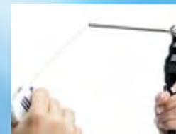
Lightly dampen a cotton swab with Hawkeye lens cleaner, isopropyl alcohol or acetone. Hawkeye lens cleaner works well on fingerprints and dust... use acetone on oil or grease. Gently clean the lens window with the fewest strokes necessary. Lightly wipe with a dry swab to eliminate smearing.
