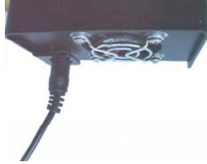
Make sure the power supply's AC cord is attached, then plug the AC cord into a 100/240V – 60/50hz AC outlet.
