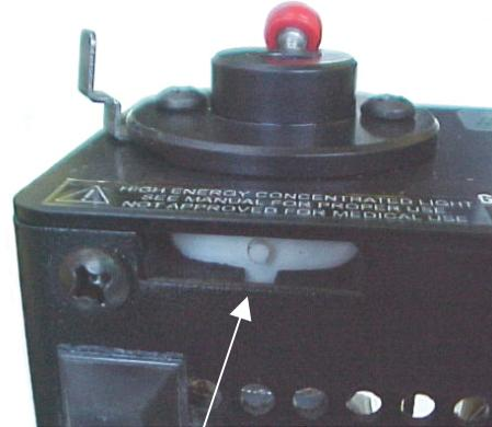
Properly seated lamp. Locating pin has passed completely through slot.
